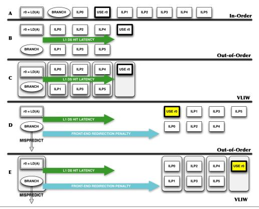
Figure 4. Misprediction recovery latency covers L1-hit latency
