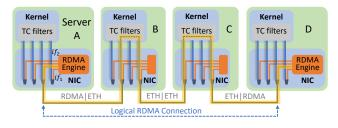
Figure 29: Host-based RDMA forwarding to create a logical RDMA connection between end hosts.
