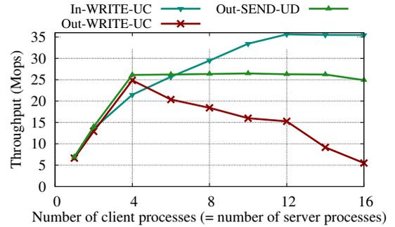
**Figure 6: Comparison of UD and UC for all-to-all communication with 32 byte payloads.** Inbound WRITES over UC and outbound SENDs over UD scale well up to 256 queue pairs. Outbound WRITES over UC scale poorly. All operations are inlined and unsignaled.
