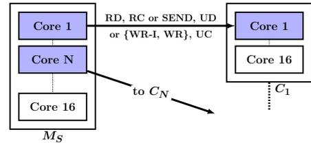
(a) Setup for measuring outbound throughput. Each server process communicates with only one client process.
