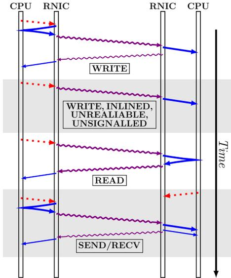
**Figure 1: Steps involved in posting verbs.** The dotted arrows are PCIe PIO operations. The solid, straight arrows are DMA operations: the thin ones are for writing the completion events. The thick wavy arrows are RDMA data packets and the thin ones are ACKs.
