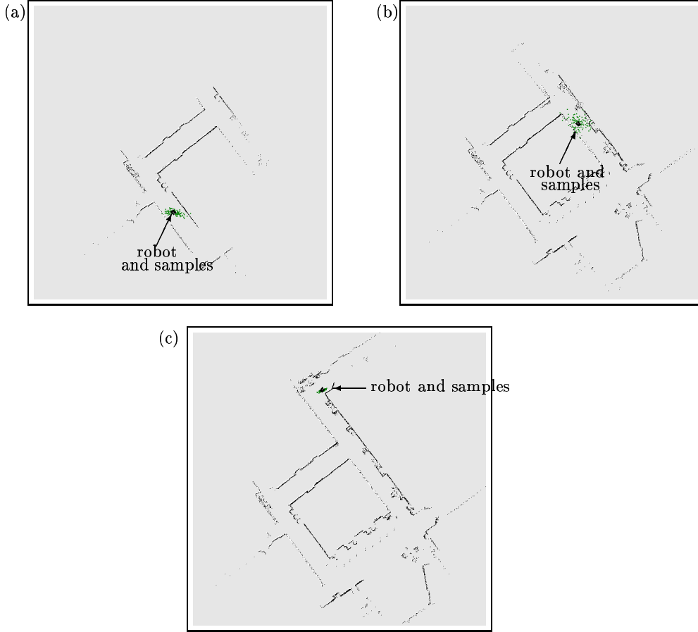
Figure 7: Incremental algorithm for concurrent mapping and localization. The dots, centered around the robot, indicate the posterior belief which grows over time (a and b). When the cycle is closed as in (c), the posterior becomes small again.
