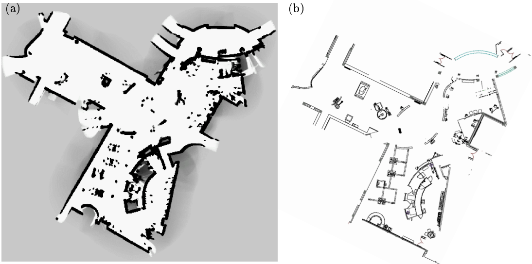
Figure 13: (a) Occupancy grid map and (b) architectural blueprint of a recently constructed museum in San Jose. Notice that the blueprint is inaccurate in certain places.
