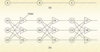
Triple modular redundancy. For each voter, if two or three of the inputs are the same, the output is equal to the input. If all three inputs are different, the output is undefined.
