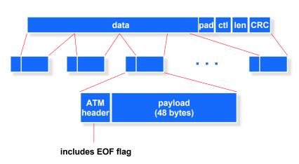
Pertinent part: Packets are spread across multiple ATM cells. Each packet is delimited by EOF flag in cell.
