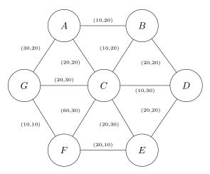
a) Given this network topology, what path gives the lowest possible end-to-end latency from node B to node F?
