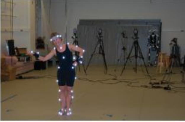
**Figure 3: A subject wearing a retro-reflective marker set in the CMU motion capture laboratory.**
