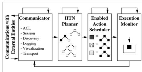
**Fig. 2.** Schematic diagram of the RETSINA Agent Architecture. The boxes represent concurrent threads and the arrows represent control and data flow. The “external entities” may be agent or non-agent software components.
