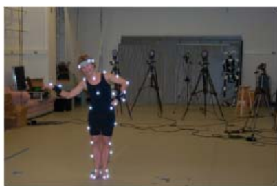
Figure 1. A subject wearing a retro-reflective marker set in the CMU Motion Capture Laboratory.
