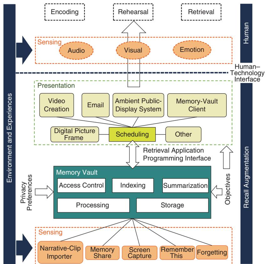
FIGURE 3. The RECALL memory-augmentation architecture.
