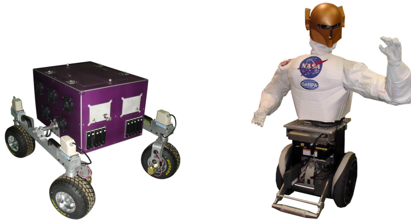
Figure 4. Left, the K-10 rover (NASA Ames) is a low-cost rover designed to operate at human interaction speeds; right, Robonaut-B (NASA JSC) is a mobile manipulation system attached to a Segway RMP differential-drive base.
