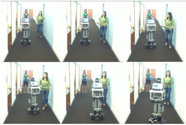
Fig. 2. CoBot robot following oscillating pathway down a hallway with in a shared environment with people.
