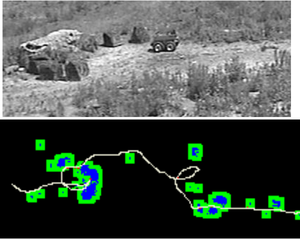
Fig. 7 Results from a field trial (above) Bullwinkle negotiates a cul-de-sac with no prior knowledge of the environment. (below) Final map created by Dstar after a 60 m traverse.
