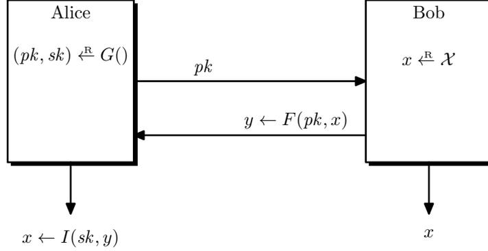
**Figure 10.1:** Key exchange using a trapdoor function scheme
