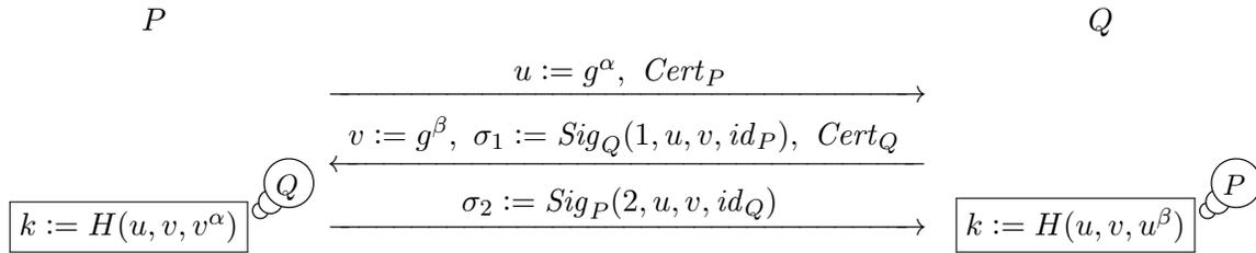
**Figure 21.6:** Protocol  $\text{AKE3}_{\text{eg}}$
