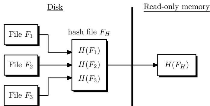
**Figure 8.2:** File integrity using small read-only memory
