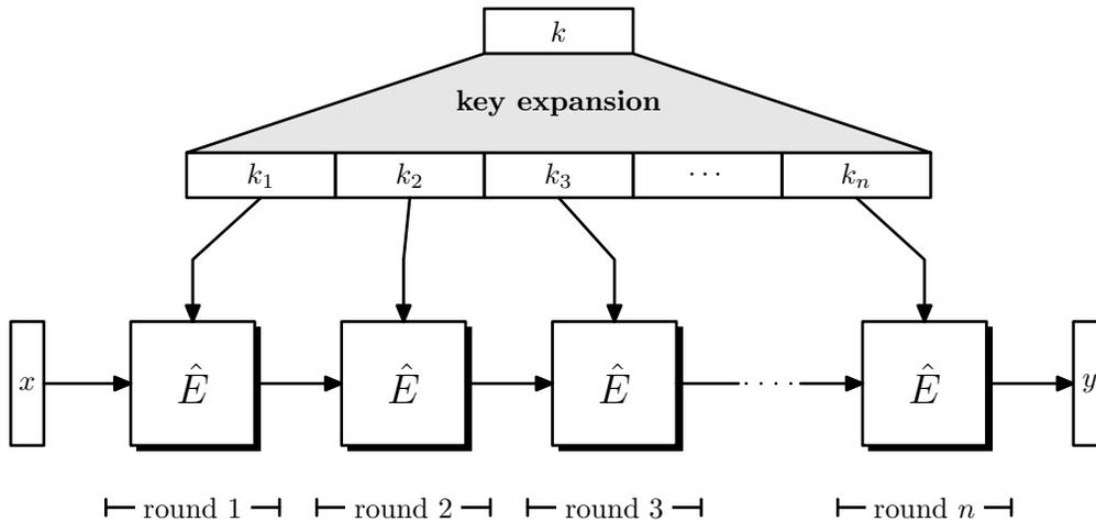
**Figure 4.6:** Encryption in a real-world block cipher
