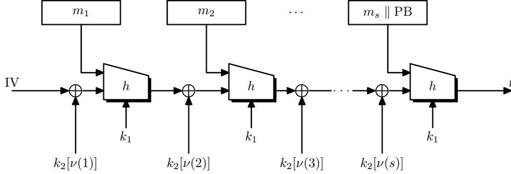
**Figure 8.15:** Extending the domain of a TCR hash
