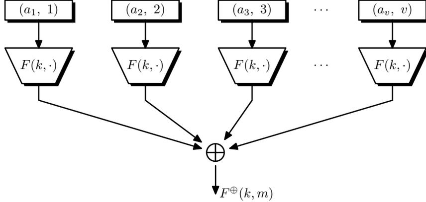
**Figure 7.2:** A parallel UHF from a small PRF
