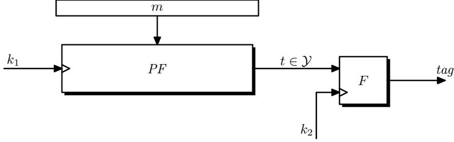
**Figure 6.4:** The encrypted PRF construction  $EF(k, m)$
