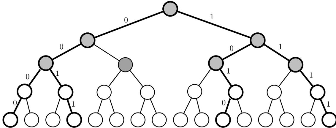
**Figure 4.16:** Evaluation tree for Hybrid 2 with  $\ell = 4$ . The shaded nodes are assigned random labels, while the unshaded nodes are assigned derived labels. The highlighted paths correspond to inputs 0000, 0011, 1010, and 1111.
