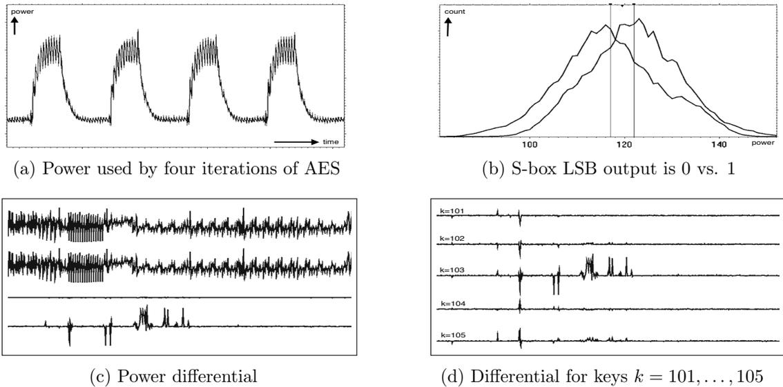
**Figure 4.12:** AES differential power analysis (source: Kocher et al. [77])
