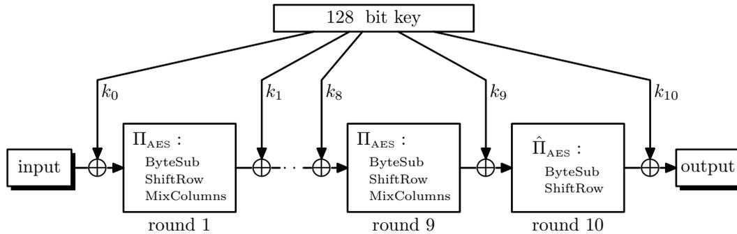
**Figure 4.11:** Schematic of the AES-128 block cipher
