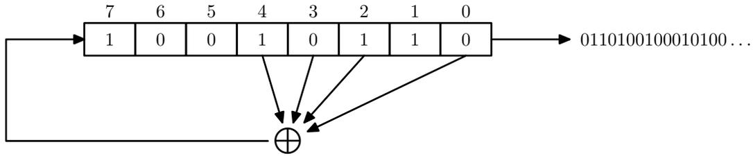
**Figure 3.10:** The 8 bit linear feedback shift register  $\{4, 3, 2, 0\}$
