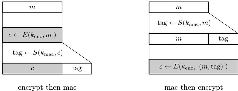
**Figure 9.1:** Two methods to combine encryption and MAC
