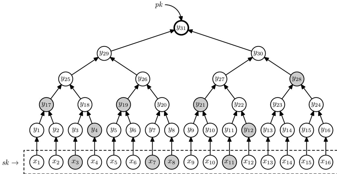
The HORST system with  $n = 16$  and  $\ell = 4$ . When  $P_{\text{hors}}(M) = \{3, 7, 8, 11\}$  the signature is the set of shaded nodes. The secret key  $sk$  is a short PRF key from which  $x_1, \dots, x_{16} \in \mathcal{X}$  are derived.
