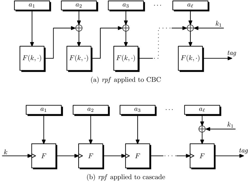
**Figure 6.6:** Secure PRFs using random prefix-free encodings
