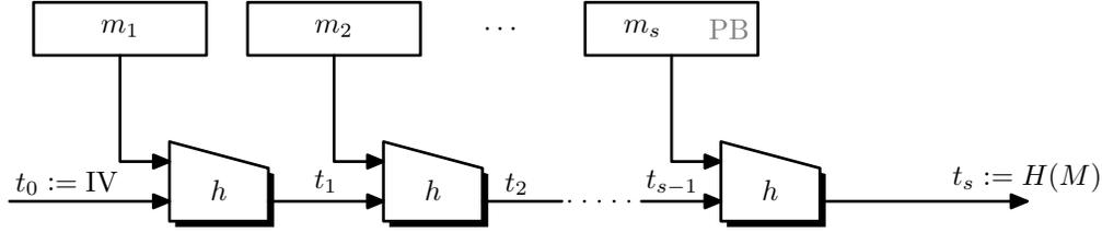
**Figure 8.5:** The Merkle-Damgård iterated hash function
