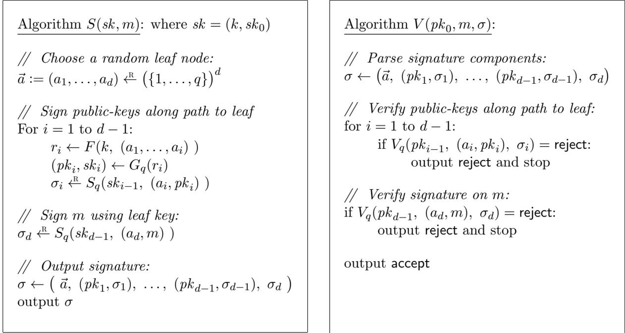
**Figure 14.7:** The Merkle signing and verification algorithms
