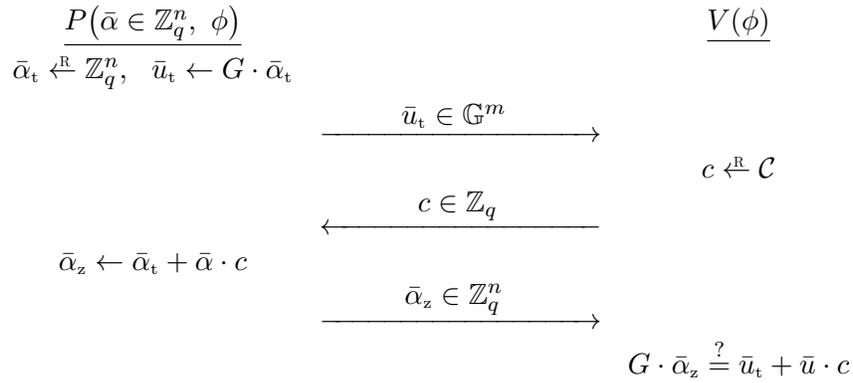
**Figure 19.9:** The generic linear protocol using matrix notation
