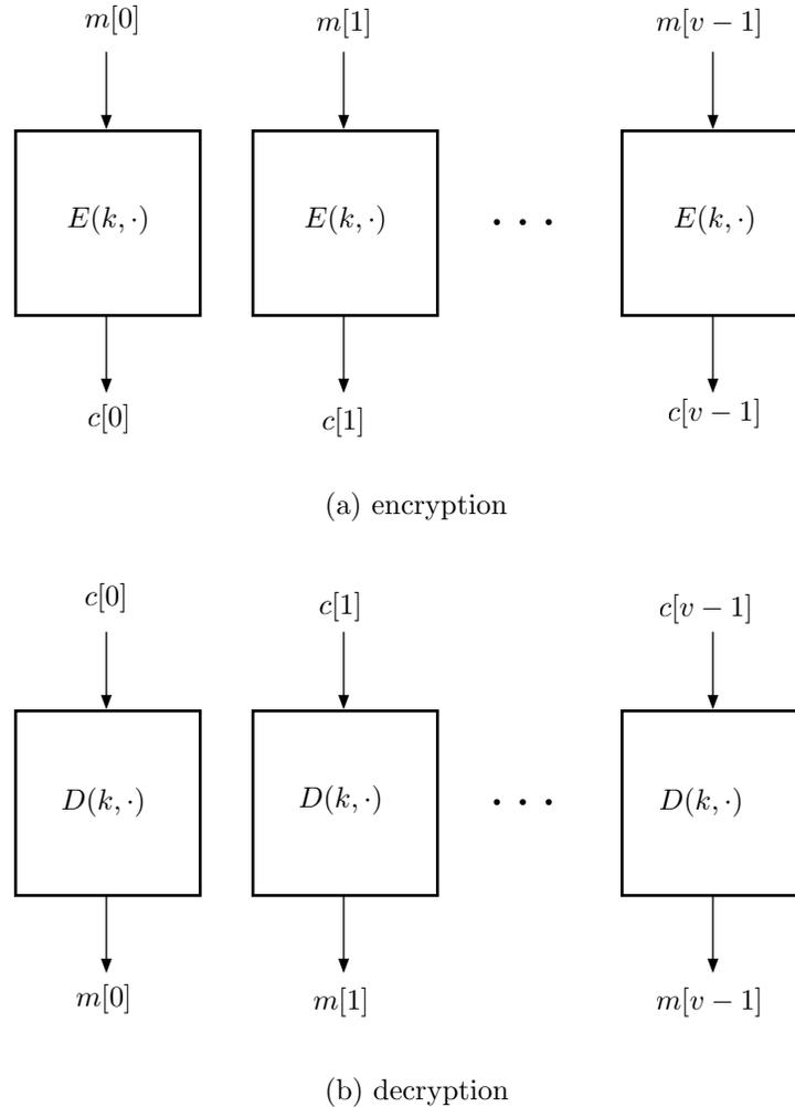
**Figure 4.4:** Encryption and decryption for ECB mode
