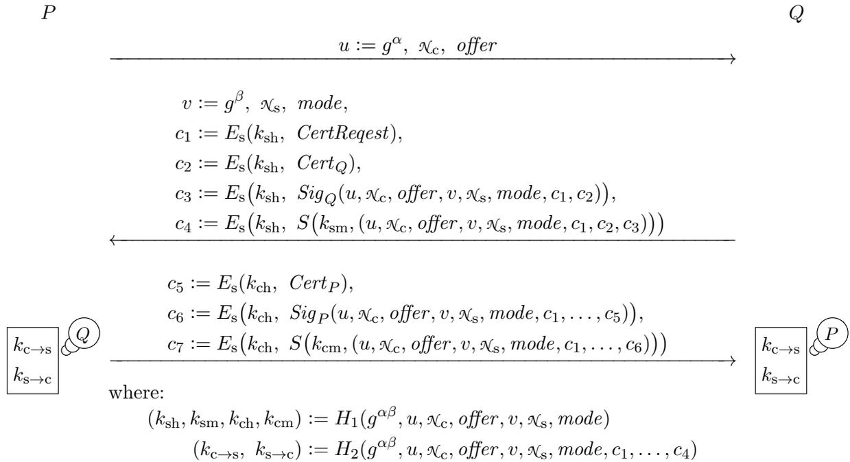
**Figure 21.12:** The TLS 1.3 key exchange protocol
