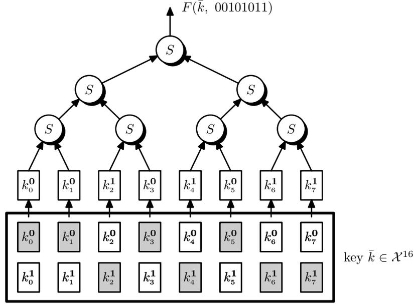
**Figure 4.18:** A PRF built from a synthesizer  $S$ . The PRF input in  $\{0,1\}^n$  is used to select  $n$  components from the key  $\bar{k} \in \mathcal{X}^{2n}$ . The selected components, shown as shaded squares, are used as shown in the figure.
