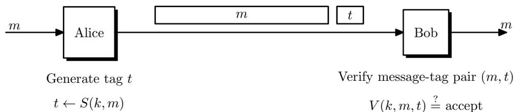
**Figure 6.1:** Short message integrity tag added to messages
