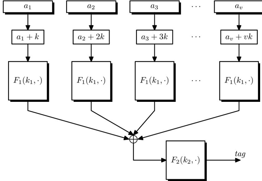
**Figure 6.9:**  $\text{PMAC}_0$  construction
