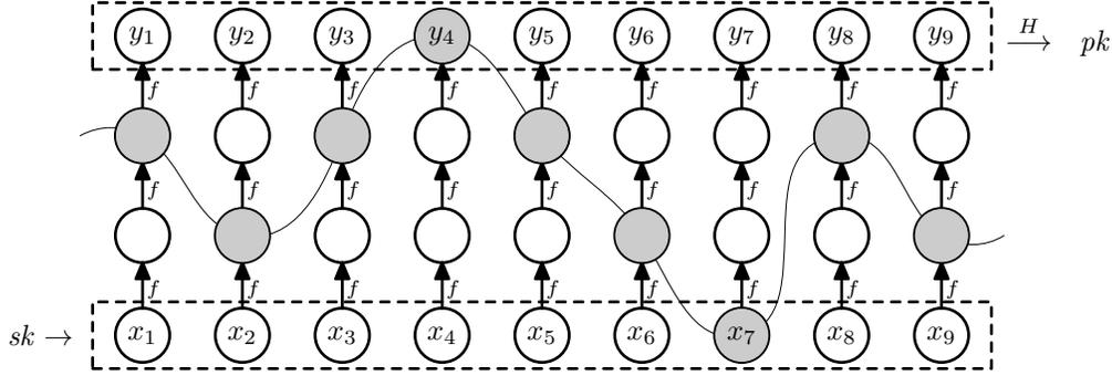
The secret key  $sk$  is used to derive  $x_1, \dots, x_9 \in \mathcal{X}$ . The public key  $pk$  is the hash of  $y_1, \dots, y_9 \in \mathcal{X}$ . The shaded circles represent the signature on a message  $m$  where  $P(m) = (2, 1, 2, 3, 2, 1, 0, 2, 1)$ . This  $P(m)$  describes a cut through the rectangle illustrated by the thin line.
