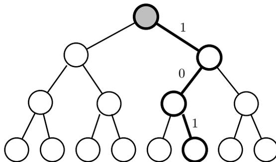
**Figure 4.15:** Evaluation tree for  $\ell = 3$ . The highlighted path corresponds to the input  $x = 101$ . The root is shaded to indicate it is assigned a random label. All other nodes are assigned derived labels.
