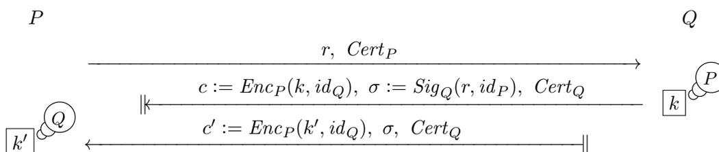
In the diagram, we write  $\llcorner$  to indicate a message blocked by the adversary, and  $\llcorner$  to indicate a message generated by the adversary. At the end of the attack,  $Q$  is holding the session key  $k$ , which is unknown to the adversary; however,  $P$  is holding the session key  $k'$ , which is known to the adversary.
