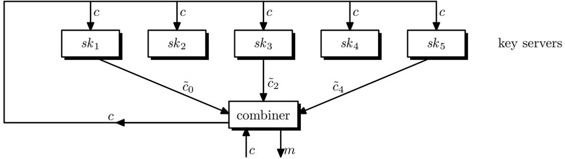
The combiner sends the given ciphertext  $c$  to all five key servers. Three servers respond, enabling the combiner to construct and output the plaintext message  $m$ .
