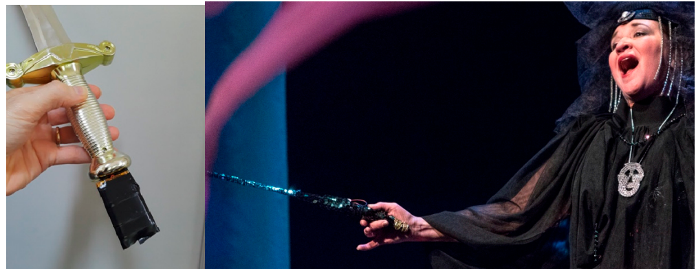
Figure 4. The sword prop and “magic wand” used in the opera production. Each has a 9 DOF sensor and microcontroller with Wi-Fi to communicate with a computer running Soundcool. Performers’ gestures trigger and control sound effects in real time.
