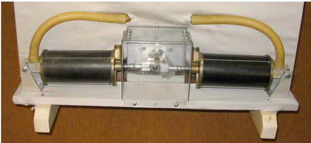
**Figure 2. The McBlare air compressor. Electric motor (not visible) drives eccentric (center) through a gearbox. Eccentric drives two air pump cylinders (right and left) in opposition.**
