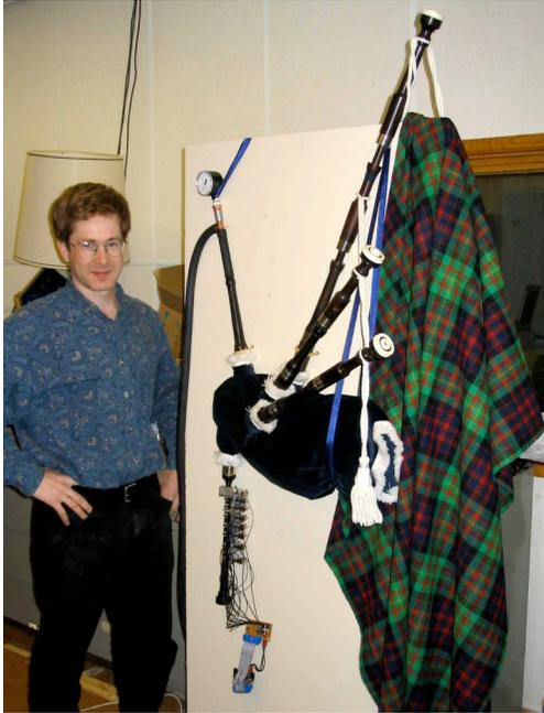
**Figure 4. Garth Zeglin with McBlare shortly before its debut at the Robotics Institute’s Twenty-Fifth Anniversary. Bagpipes are mounted on a display board that conceals the pump and additional electronics.**
