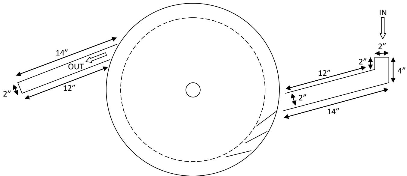
All troughs are 2" deep into page to reflect the width of the wheel
