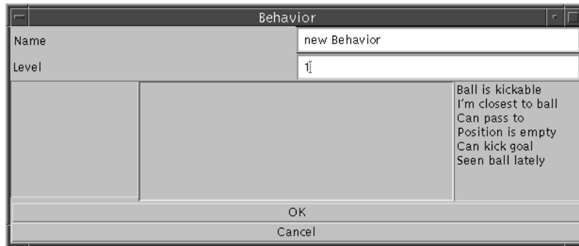
Fig. 2. The Behavior Specification Window. This is how the window appears when the New Behavior button is pressed. The list on the right shows the predicates that can be used by the behavior. The, initially empty, list on the left shows names of behaviors that can be used to implement the functionality of the behavior. The middle of the window will show selected behaviors and their associated activation parameters.
