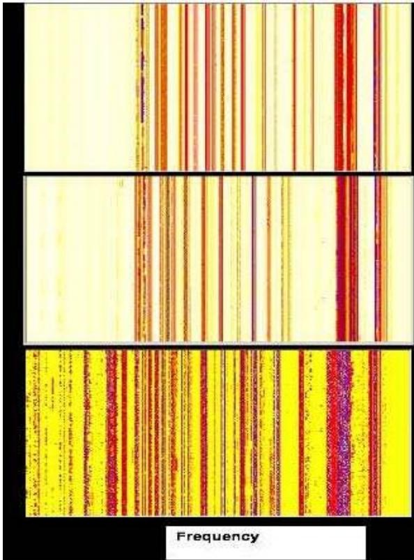
Snapshot of utilization of 700 MHz slice of spectrum below 1 GHz
