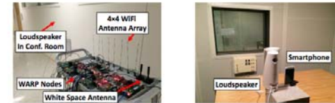
Figure 15: ART hardware platform. Test- ing ART outside a conference room.
