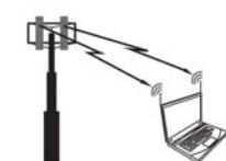
Multilayer transmission ("SU-MIMO") for higher data rates in a given bandwidth
