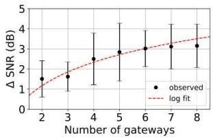
Combined signal SNR increases logarithmically
