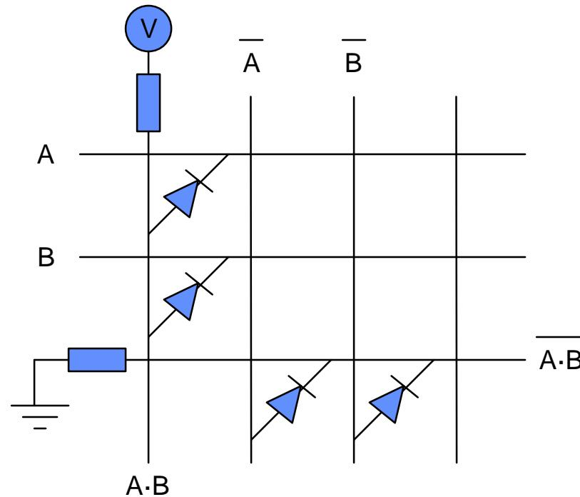
$\{\text{AND, NOT}\}$  is a functionally complete set for Boolean functions, so any Boolean function can be composed from nanoBlocks
