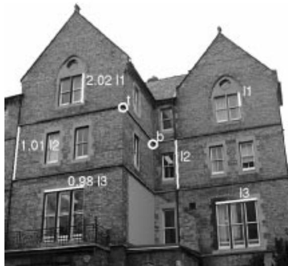
**Figure 5: Measuring the ratio of lengths of parallel line segments lying on two parallel scene planes:** The points  $t$  and  $b$  (together with the plane vanishing line and the vanishing point) define the homology between the two planes on the facade of the building.
