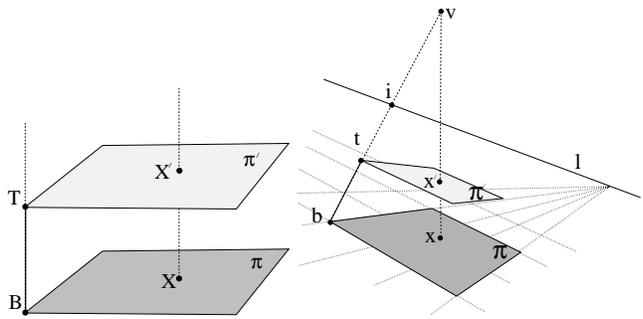
**Figure 4: Homology mapping between parallel planes:** (left) A point  $X$  on plane  $\pi$  is mapped into the point  $X'$  on  $\pi'$  by a parallel projection. (right) In the image the mapping between the images of the two planes is a homology, with  $v$  the vertex and  $l$  the axis. The correspondence  $b \rightarrow t$  fixes the remaining degree of freedom of the homology from the cross-ratio of the four points:  $v, i, t$  and  $b$ .
