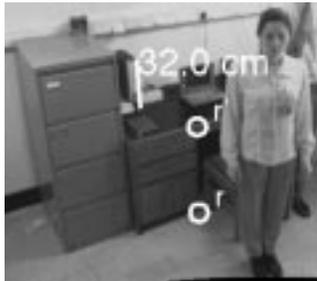
**Figure 11: Measuring heights of objects on separate planes:** Using the homology between the ground plane (initial reference) and the plane of the table, we can determine the height of the file on the table.
