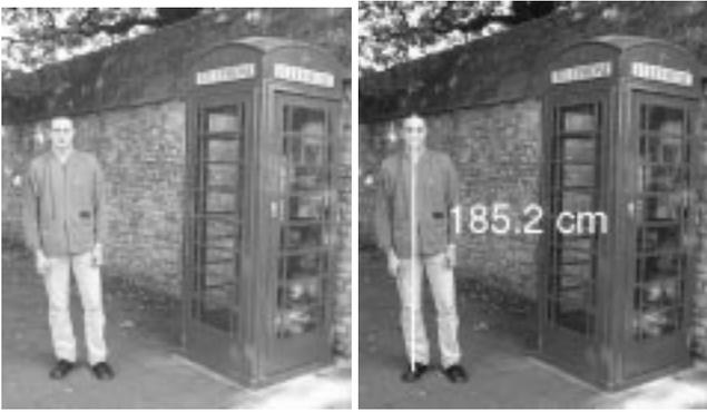
**Figure 10: Measuring the height of a person in an outdoor scene:** The ground plane is the reference plane, and its vanishing line is computed from the slabs on the floor. The vertical vanishing point is computed from the edges of the phone box, whose height is known and used as reference. The vertical height is 187cm, but note that the person is leaning slightly on his right foot.
