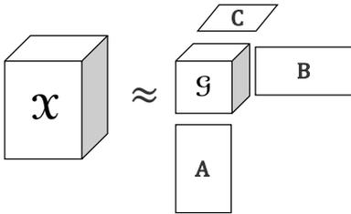
Fig. 2: Rank- $R$  Boolean Tucker decomposition of a three-way tensor  $\mathcal{X}$ .  $\mathcal{X}$  is decomposed into a binary core tensor  $\mathcal{G}$ , and three binary factor matrices  $\mathbf{A}$ ,  $\mathbf{B}$ , and  $\mathbf{C}$ .
