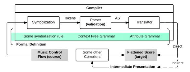
Figure 3.1: Structure of defining, validating and compiling music control flow notation
