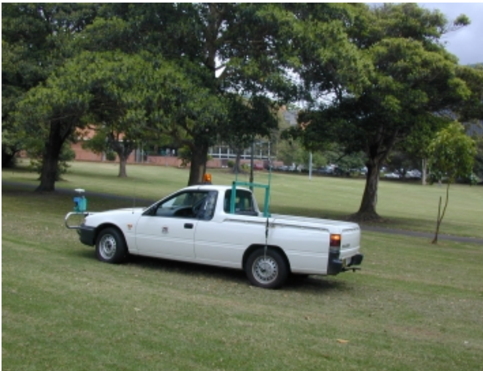
Figure 7. Utility car used for the experiments. The vehicle is equipped with a Sick laser range and bearing sensor, linear variable differential transformer sensor for the steering and back wheel velocity encoders.
