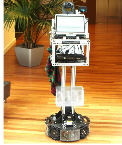
Figure 3: The CoBot mobile service robot that our approach is implemented on.
