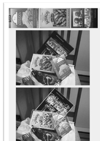
Figure 3: Model images of planar objects are shown in the top row. Recognition results below show model outlines and feature keys used for matching.
