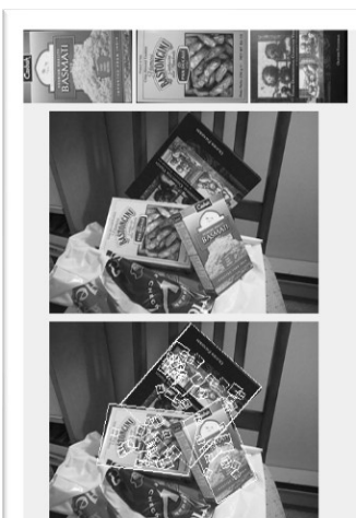
Figure 3: Model images of planar objects are shown in the top row. Recognition results below show model outlines and match keys used for matching.
