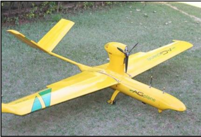
Figure 1: The ARARA aircraft. Wingspan: 3 m; Engine: two-stroke, 40 cc, 5 HP, AVGAS; max weight: 20 kg; payload: 3 kg; flight endurance: 4 h; cruise speed: 100 km/h; stall speed: 40km/h; autonomous or remote controlled; emergency parachute.
