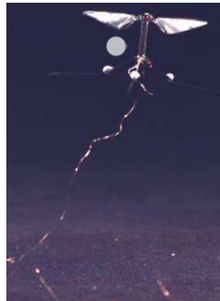
(a) A picture of a flapping-wing microbot prototype taken from (Chirarattananon, Ma, and Wood 2013).
