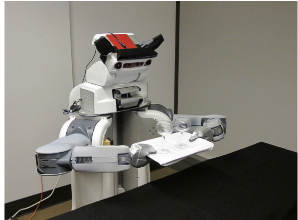
Fig. 1: The PR2 robot manipulating a tray with two wine glasses on it.
