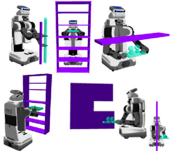
Fig. 5: Clockwise from top left: stick around a pole, wood board in bookshelf, tray with wine glasses under a table, tray with wine glasses near wall and tray with a scotch glass in bookshelf.
