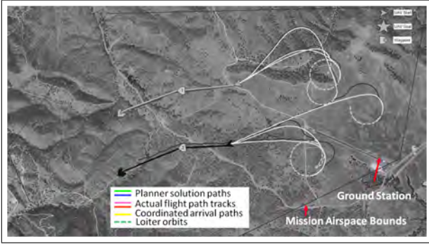
Fig. 14. Coordinated vehicle tracks to start of a planned mission from arbitrary orbit locations (acquired from flight test).
