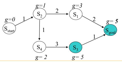
• Computes  $g^*$ -value Optional but useful optimization: If OPEN contains multiple states with the smallest g-values and  $s_{goal}$  is one of them, while  $(s_{goal}$  is not expanded and Or L. then select  $s_{goal}$  for expansion remove s with the smallest g(s) from OPEN; insert s into CLOSED; for every successor s' of s such that s' not in CLOSED
