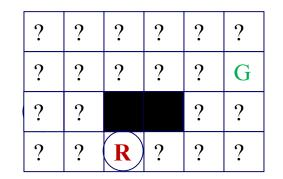
Intuition behind uninformed A\*: Starting with the start state (marked R), always compute next the state with smallest g\* value!
