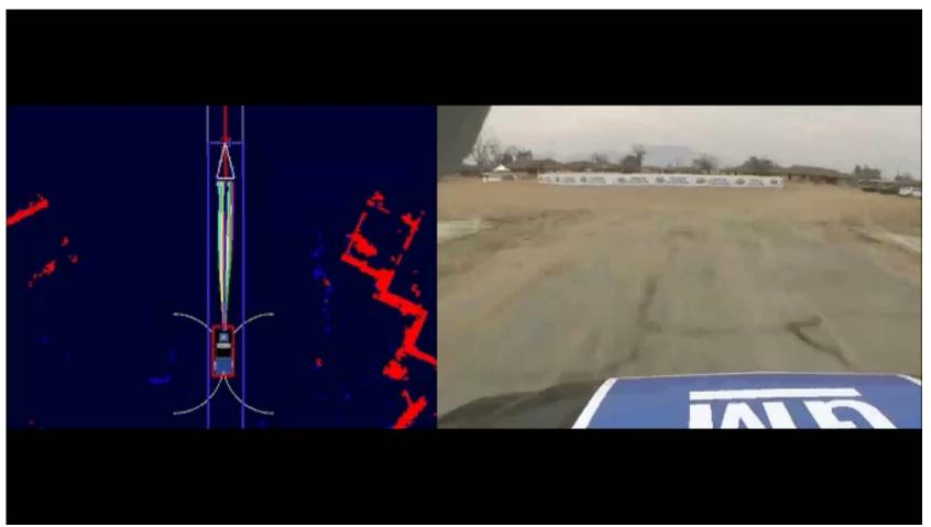
$(x,y,\Theta)$  planning with ARA\*-based algorithm on Lattice Graphs
