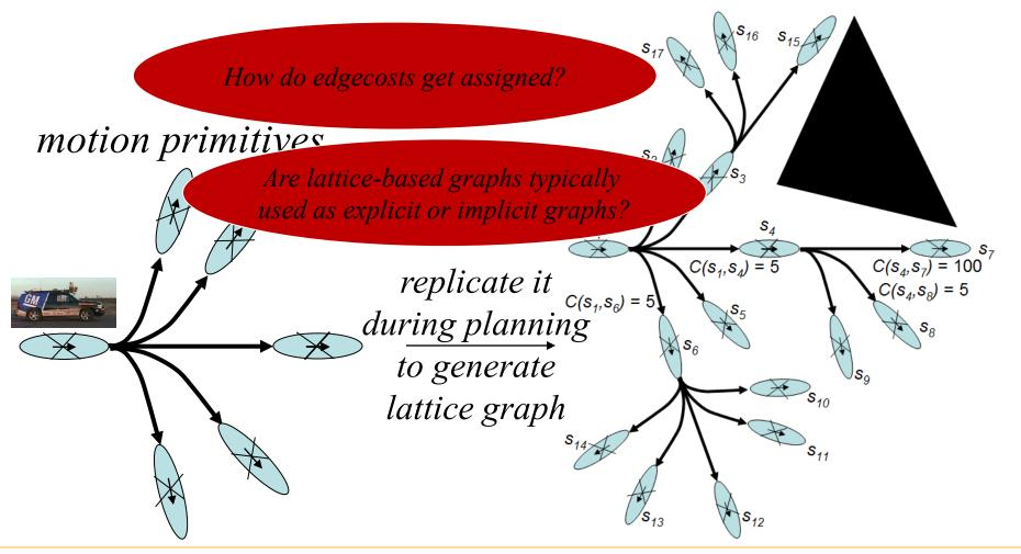
• **Board example** for  $(x, y, \Theta)$  planning for a unicycle model (minimum turning radius)
