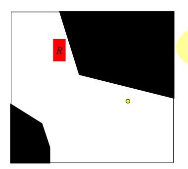
Construct a 3D grid  $(x,y,\Theta)$  assuming point robot (i.e., a cell  $(x,y,\Theta)$  is free whenever its (x,y) is free) and compute the **actual** validity of only those cells that get computed by the graph search
