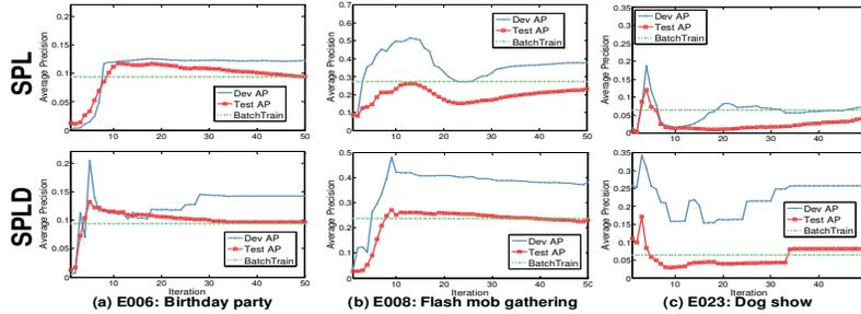
Figure 3: The validation and test AP in different iterations. Top row plots the SPL result and bottom shows the proposed SPLD result. The  $x$ -axis represents the iteration in training. The blue solid curve (Dev AP) denotes the AP on the validation set, the red one marked by squares (Test AP) denotes the AP on the test set, and the green dashed curve denotes the Test AP of BatchTrain which remains the same across iterations.
