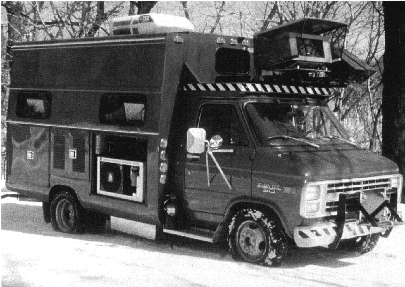
Figure 1. NAVLAB I—An autonomous vehicle, incorporating all aspects of robotics, including perception, planning, mechanisms, computing, and integration.
