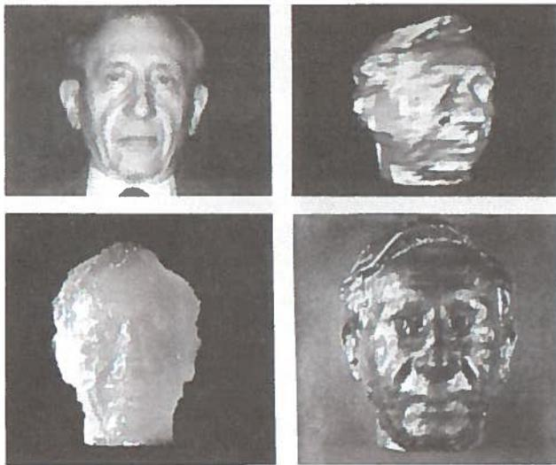
**Fig. 2** Video image of subject (upper left). Computer-aided design (CAD) model of subject created from depth measurements from a range scanning system (upper right). Stereolithography pattern created from CAD data (lower left). Sprayed 410 stainless-steel-faced sculpture (lower right)
