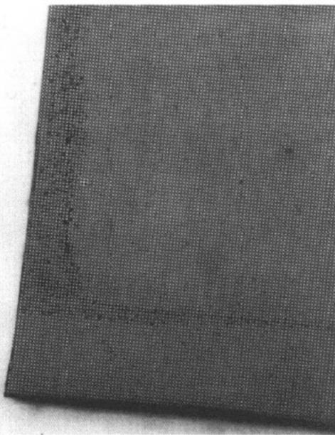
**Figure 5.** Optical micrograph of sample surface after separation. The dark (damaged) areas are regions where the microstructure tabs have broken.
