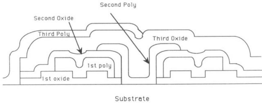
**Figure 1.** Schematic cross section of the polysilicon and SiO<sub>2</sub> layers comprising the device, before the sacrificial oxide etch.
