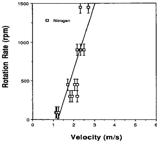
Figure 5. Rotation rate (rpm) versus nitrogen velocity ( $\text{m s}^{-1}$ ).
