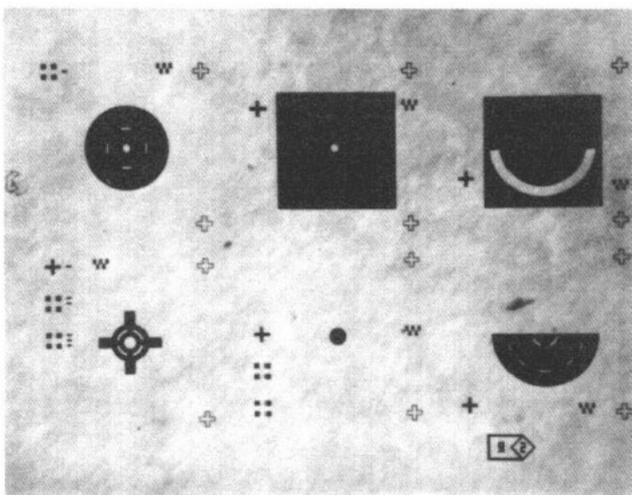
**Figure 2.** Mask patterns. The upper patterns are oxide cuts; the lower define polysilicon structures. The rotor itself is defined by the pattern in the lower left; the one in the lower right defines the semicircular cap (third polysilicon layer) which covers half the rotor.
