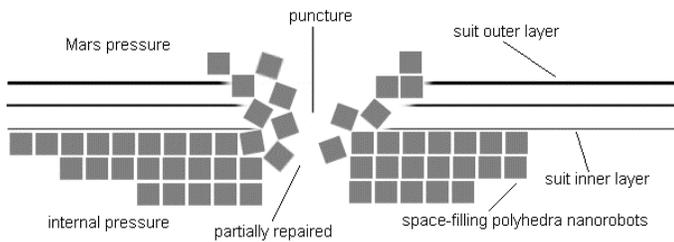
**Figure 6:** Space-Filling Polyhedral Nanorobots – *Space-filling polyhedral nanorobots rapidly converge upon damaged areas and seal them*
