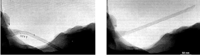
**Figure 3:** Elastic Properties of Nanotubes – *Single wall carbon nanotubes have been shown to possess extraordinary elasticity. Buckling effects are observed (arrows, left) under applied load, but there is no permanent deformation.*[6]
