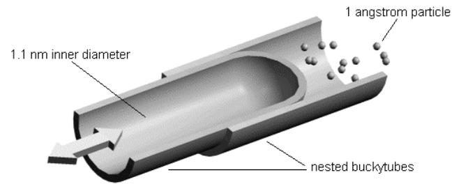
**Figure 8:** Molecular Actuator – A carbon nanotube nested in an open buckytube can serve as a molecular actuator.
