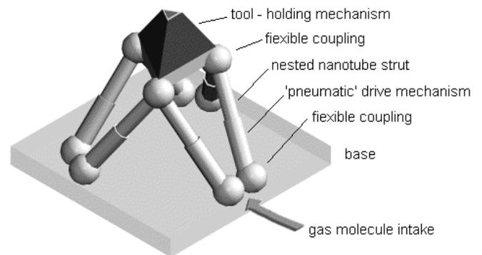
**Figure 7:** The Stewart Platform – *The Stewart platform has six 100 nm length struts, which provide six degrees of positional freedom to the manipulator tip.*
