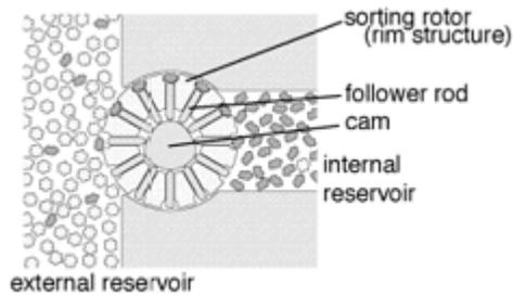
**Figure 11:** Sorting Rotor – Variable affinity binding sites on a rotor make it possible to separate fuel and other molecules out of the feedstock. Operated in reverse, they can dispose of wastes.[23]
