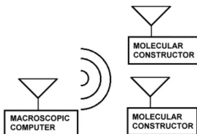
**Figure 5:** Broadcast Architecture – In a broadcast architecture, many molecular constructors are under the complete control of a single macroscopic computer.[5]
