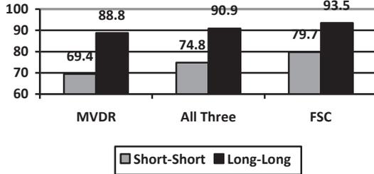
Figure 7: Improvement due to FSC for the best single-feature-type system (MVDR) and the combined system with all three front-end features under mismatched condition
