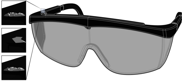
Fig. 11. These glasses have tiny details in the input geometry, which we can resolve with a large max depth for our BSP tree ( top left ). If we use a low max depth, these details get simplified into a few regions ( middle left ). However, if we aggressively split along separating lines, we lose our ability to simplify regions, even at the same low max depth ( bottom left ).
