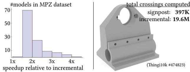
Fig. 23. Even for basic tasks like finding crossings for an intrinsic Delaunay triangulation, our data structure is faster than the incremental overlay of Fisher *et al.* (left). In extreme cases, the incremental scheme may compute far more crossings than are actually needed for the final overlay (right).
