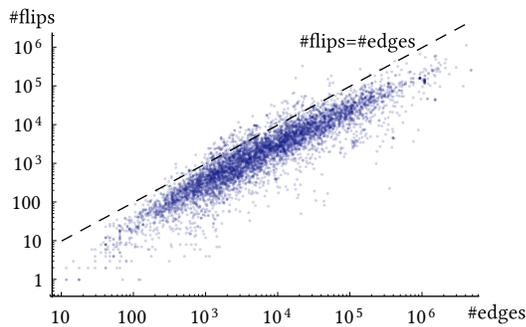
Fig. 10. By running the Delaunay edge flipping algorithm on a large data set we observe a surprising trend: the number of flips required in practice is rarely more than the number of edges in the input mesh. Here each blue dot represents a mesh from the *Thing10k* dataset.
