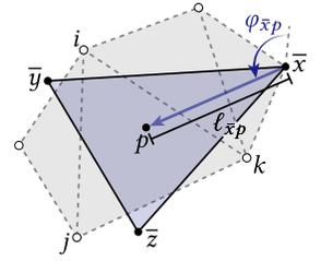
**3.4.2 Overlay Extraction.** If an overlay mesh is needed, we first perform a tracing query along each intrinsic edge  $ij \in E$ , and store a sorted list of barycentric coordinates  $t \in [0, 1]$  where  $ij$  crosses an extrinsic edge (marked by “ $\times$ ” in the figure below). For each intrinsic triangle  $ijk$ , we emit a collection of extrinsic triangles and quads; there are just two cases to consider (illustrated inset below):
