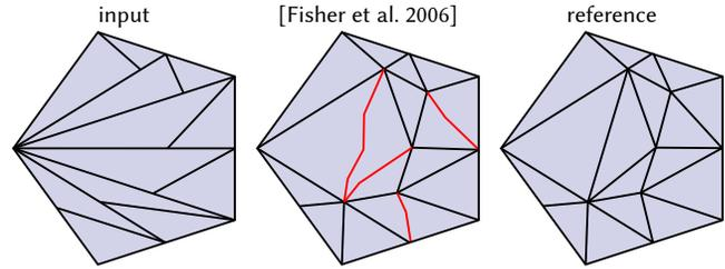
Fig. 27. Even though the incremental overlay of Fisher *et al.* guarantees topological correctness, it can still yield geometrically inaccurate edges—as shown here for the Delaunay triangulation of a near-degenerate input.
