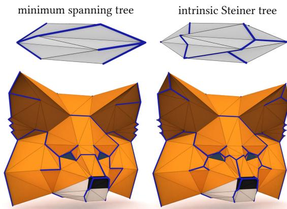
Fig. 15. Our data structure allows planar computational geometry algorithms to be easily translated into the polyhedral setting. Here we apply a classic Euclidean algorithm for *Steiner tree approximation* to find shorter cuts through polyhedral surfaces.
