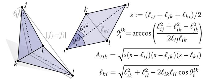
Fig. 9. *Left*: when working with an intrinsic triangulation, the length  $\ell_{ij}$  of an edge will in general be different from the extrinsic distance  $|f_j - f_i|$  between its endpoints. *Right*: instead, quantities like triangle areas  $A_{ijk}$  and interior angles  $\theta_i^{jk}$  can be easily computed from the intrinsic edge lengths.
