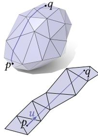
Algorithmically, each vertex of the path is found by computing 2D ray-line intersections with the edges of the current triangle, and moving to the closest intersection point. The direction of the ray is then transformed into the coordinate system of the next triangle (by constructing a vector that makes the same angle with the shared edge), and the process is repeated. The final output is the barycentric coordinates of the point  $q$ , as well as a pointer to the triangle containing  $q$ .
