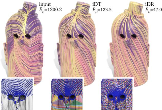
Fig. 21. Our signpost data structure is also well suited for tangent vector field processing. Here we draw streamlines of the vector field with smallest Dirichlet energy  $E_D$  (showing vectors in the inset); using an intrinsic triangulation yields a much smoother field.
