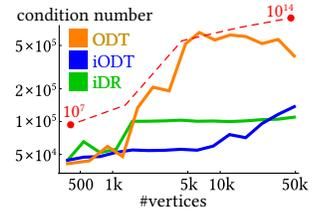
Fig. 17. Condition number for FEM Laplacian with different triangulations; values for regular 4-1 refinement (red) are off the chart.
