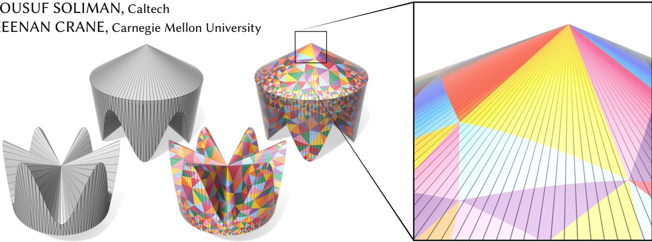
Fig. 1. Our data structure makes it possible to treat a crude input mesh (*left*) as a high-quality *intrinsic triangulation* (*right*) while exactly preserving the original geometry. Existing algorithms can be run directly on the new triangulation as though it is an ordinary triangle mesh. Here, a mesh with tiny input angles becomes a geometrically identical Delaunay triangulation with angles no smaller than  $30^\circ$ —a feat impossible for traditional, extrinsic remeshing.
