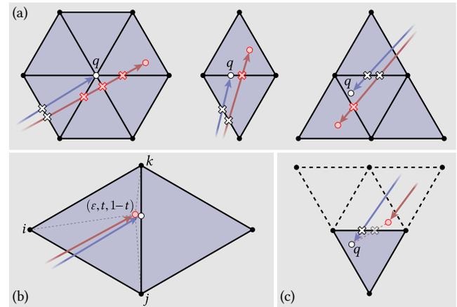
Fig. 28. Even on a nice mesh, a naïve tracing query from  $p$  to  $q$  may generate spurious crossings (in red) due to floating point error. Our robust tracing procedure helps provide reliable behavior even on highly degenerate models.
