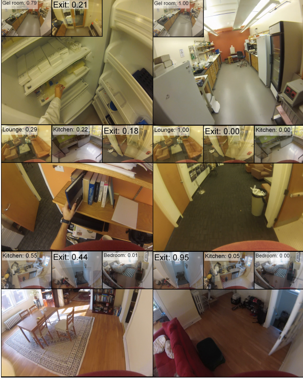
Figure 6: Goal forecasting examples: A temporal sequence of goal forecasting results is shown in each row from left to right, with the forecasting destination icons, labels, and probabilities inset sorted by probability. Top: the scientist acquires a sample to boil in the gel room. Middle: the user acquires a textbook and travels to the lounge to read. Bottom: the user leaves their apartment.
