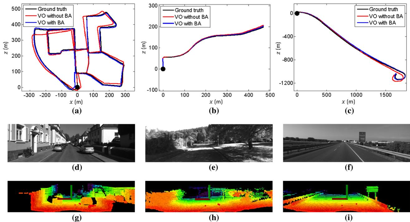
**Fig. 11** Sample results of the proposed method using the KITTI datasets. The datasets are chosen from three types of environments: urban, country, and highway from left to right. In **a–c**, we compare results of the method with and without the bundle adjustment, to the GPS/INS ground truth. The *black dots* are the starting points. An image
