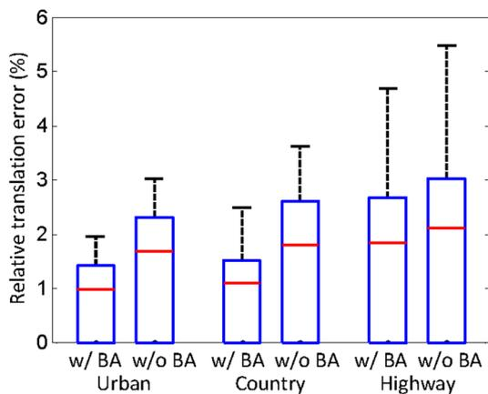
**Fig. 13** Comparison of relative translation errors in urban, country, and highway environments, tested with the KITTI datasets. In each environment, we compare errors with and without the bundle adjustment. The *black*, *blue*, and *red* lines indicate 100, 75 %, and median of the errors (Color figure online)
