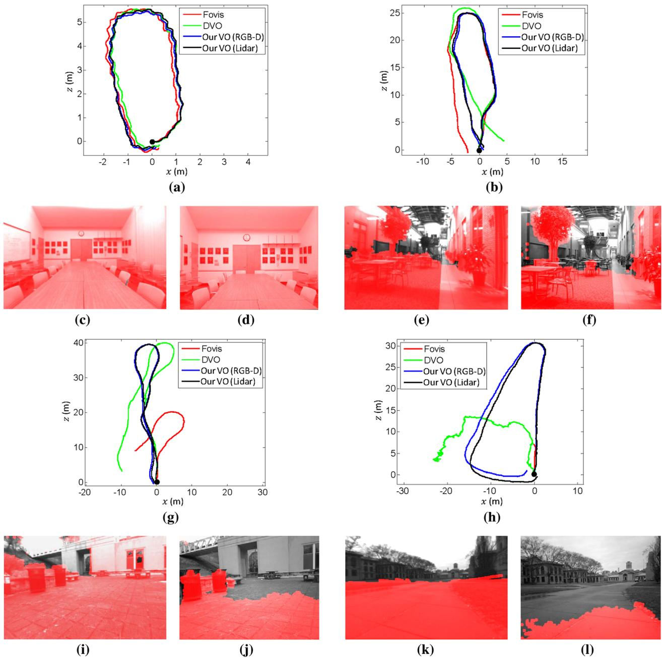
**Fig. 9** Comparison of four methods using author-collected datasets: Fovis, DVO, and two versions of our method using depth from an RGB-D camera and a lidar. The environments are selected respectively from a conference room (a, c, d), a large lobby (b, e, f), a clustered road (g, i, j), and a flat lawn (h, k, l). We present two images from each dataset. The
