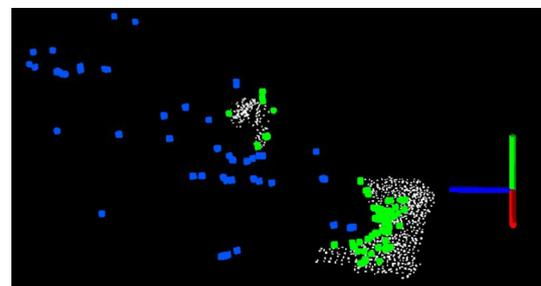
**Fig. 7** Features projected into the 3D environment corresponding to Fig. 1. The depth map (*white dots*) is from depth images collected by the RGB-D camera in Fig. 2a, only available within a limited range. The *green dots* are features whose depth is provided by the depth map, and the *blue dots* are from triangulation using the previously estimated motion (Color figure online)
