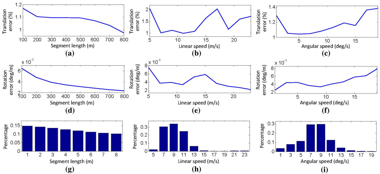
**Fig. 12** Analysis of accuracy with the KITTI datasets. On the *top* and *middle* rows, we show translation and rotation errors, by averaging errors in the 11 datasets listed in Table 2. The translation errors are represented as fractions of the distance traveled, using data segments in
