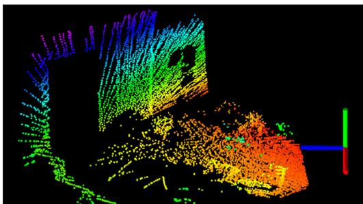
**Fig. 5** An example of the depth map with point clouds perceived by the lidar in Fig. 2b. The *points* are color coded by elevation. The camera points to a wall during data collection
