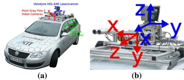
**Fig. 10** **a** Vehicle used by the KITTI benchmark for data logging. The vehicle is mounted with color stereo cameras, monochrome stereo cameras, a Velodyne lidar, and a high accuracy GPS/INS for ground truth acquisition. Our method uses data from a single camera and the Velodyne lidar for motion estimation. **b** shows a zoomed in view of the sensors (Color figure online)
