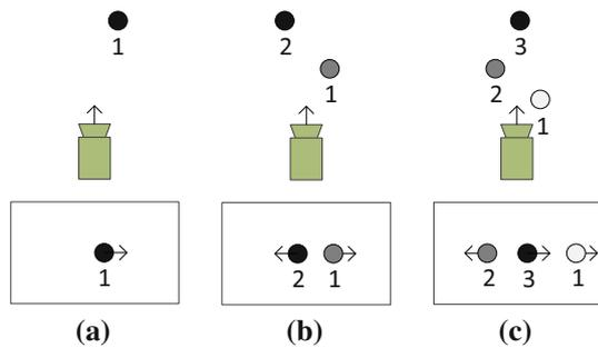
**Fig. 4** Illustration of depth map registration. **a–c** represent three image frames. In each figure, we show the camera frame on the *top* and the corresponding image on the *bottom*. Three points are registered labeled with 1–3. The illumination of a point indicates its distance to the camera. In this example, the camera moves forward. The registered points change illumination during the camera motion, leave the camera field of view in the end and are removed from the depth map
