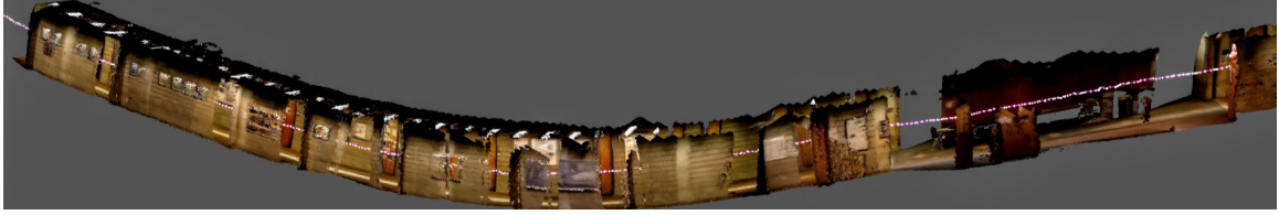
(a) Kintinuous/RGBD SLAM [40] generates a map that bends.
