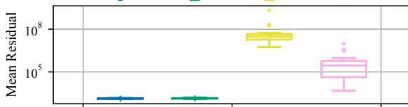
Fig. 3: Comparison of MESA variants derived from Geodesic (●), Split (■), Approximate-Geodesic (▲) and Chordal (▽) constraints on 20 synthetic 3D pose graph datasets. Split and Geodesic constraints significantly outperform the alternatives.
